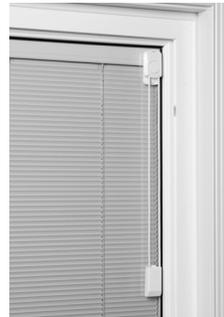
2 Position the cord tensioner, keeping the cord in tension. The operator tip on the cord tensioner should be positioned at approximately the line on the tensioner or slightly higher to keep the cord engaged. Excessive tension on the loop will hinder cord movement. (Photo #22)
