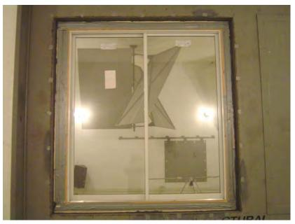
Source Room View of Installed Specimen
