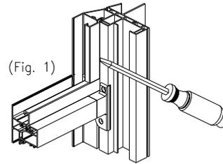
**Step 1.** Using a flat head screwdriver, remove the vertical glazing beads from the fixed panel. (Fig. 1)
