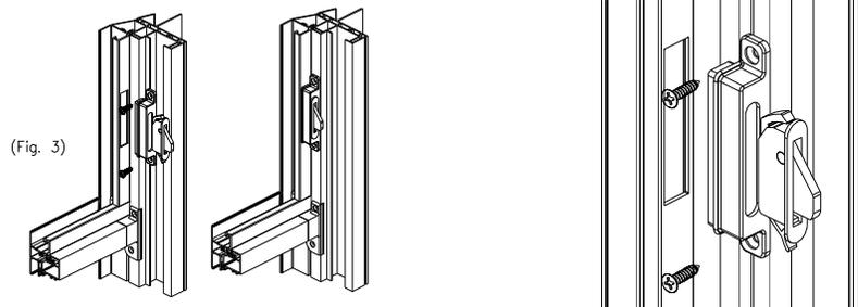
**Step 5.** After the WOCD assemblies are secured to both jambs, confirm proper installation by raising the sash. The WOCD should restrict the sash from opening fully and no space should exist at the lowest portion of the window opening that would permit the passage of a rigid sphere measuring 4.0 inches in diameter. Close the sash.
