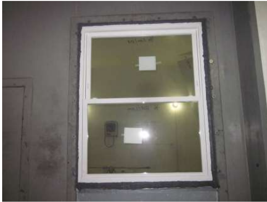
Receive Room View of Installed Test Specimen
