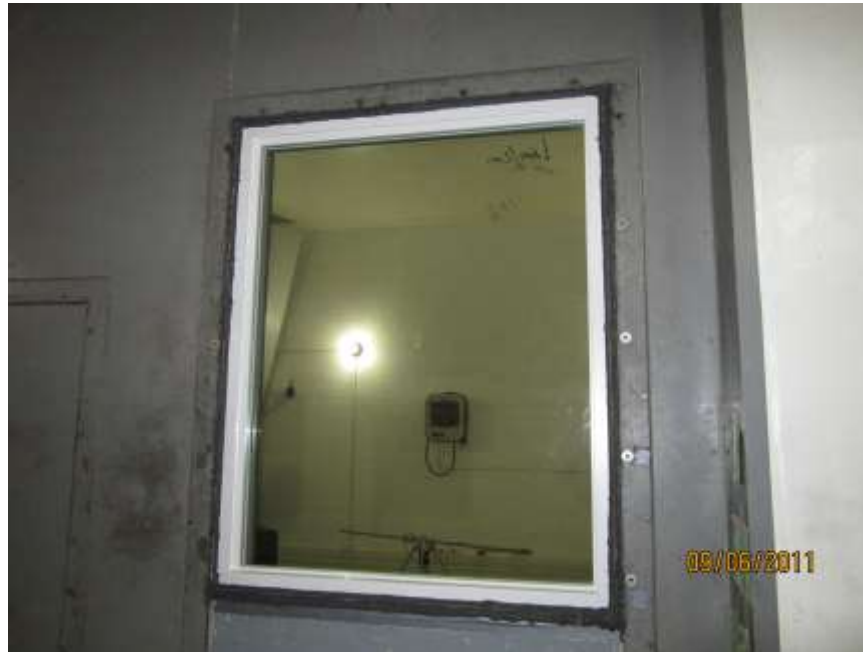
Receive Room View of Installed Test Specimen
