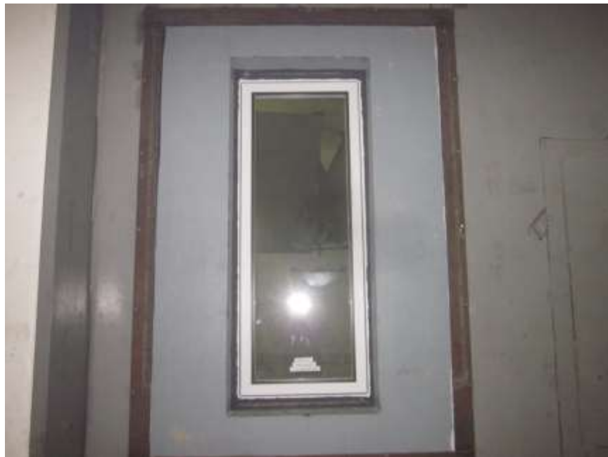
Source Room View of Installed Test Specimen
