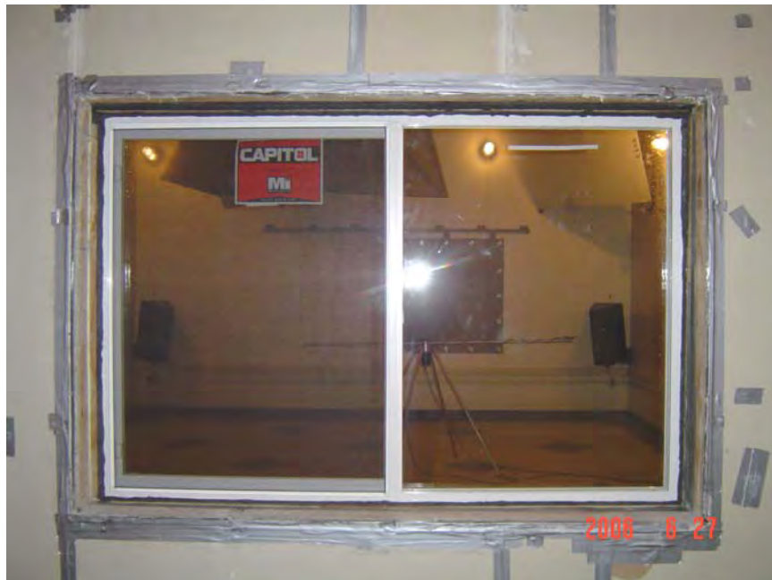
View of Specimen Installed in Source Room
