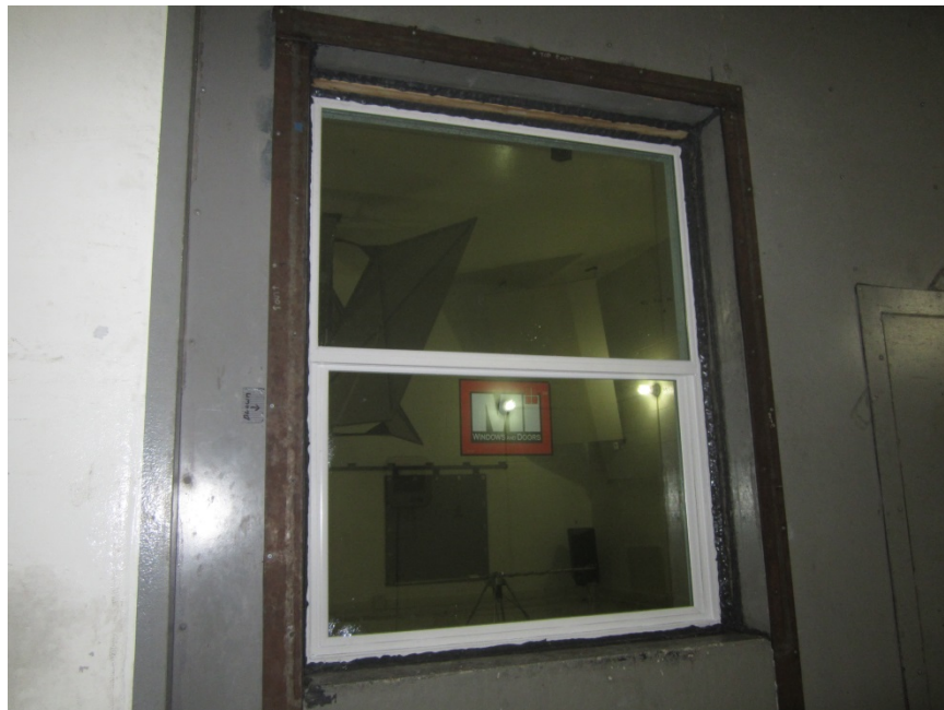
Source Room View of Installed Specimen
