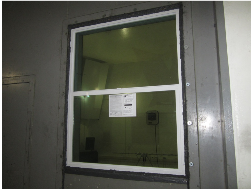
Receive Room View of Installed Specimen
