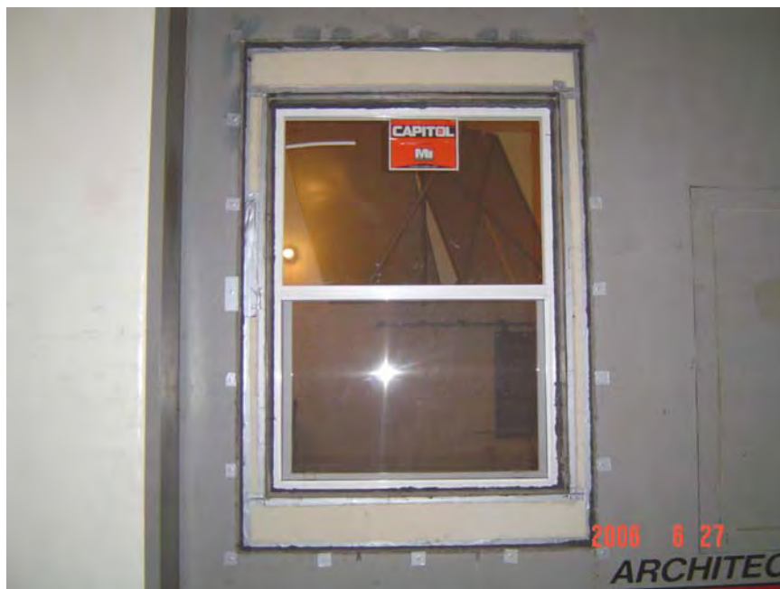
View of Specimen Installed in Source Room
