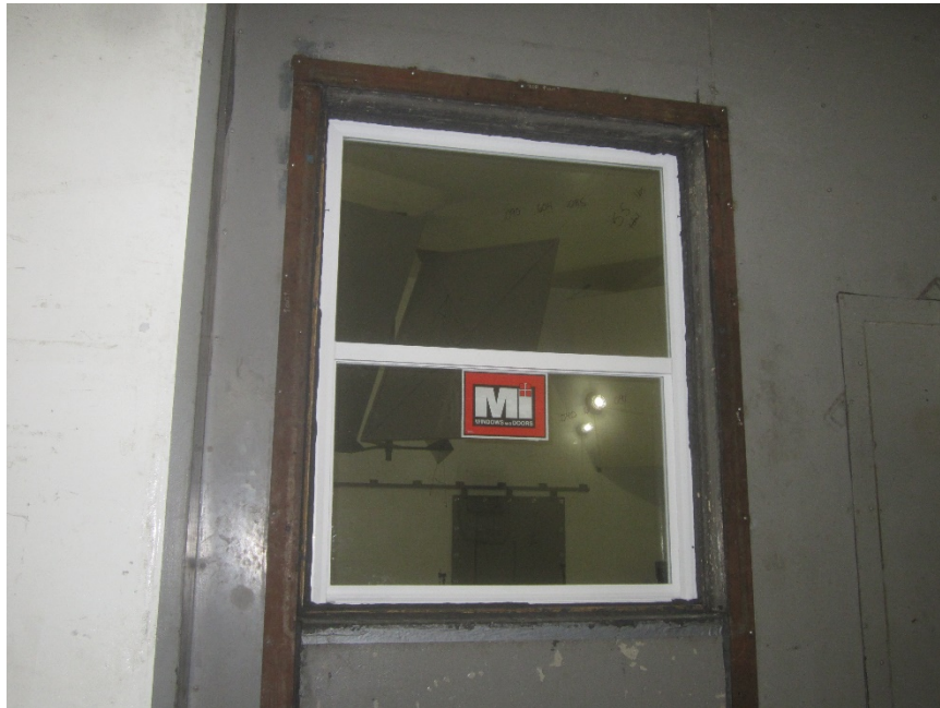
Source Room View of Installed Test Specimen
