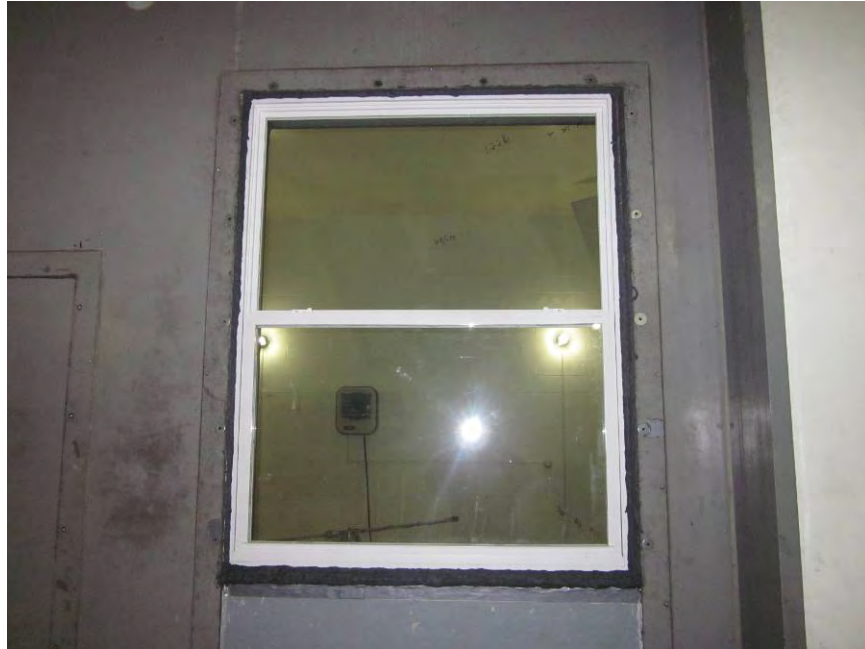
Receive Room View of Installed Specimen
