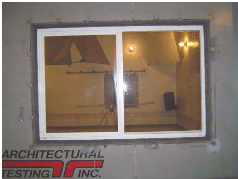
Source Room View of Installed Specimen
