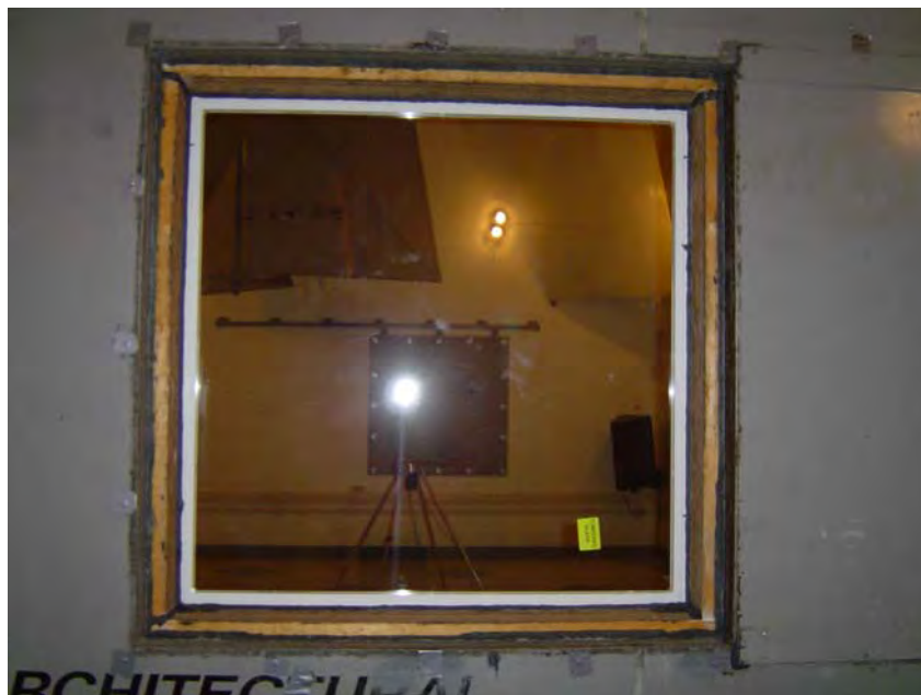
Sample Installed in Test Chamber, Source Room View
