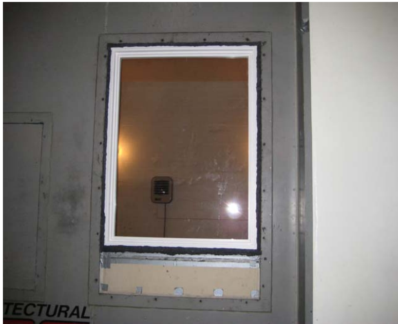
Sample Installed in Test Chamber
