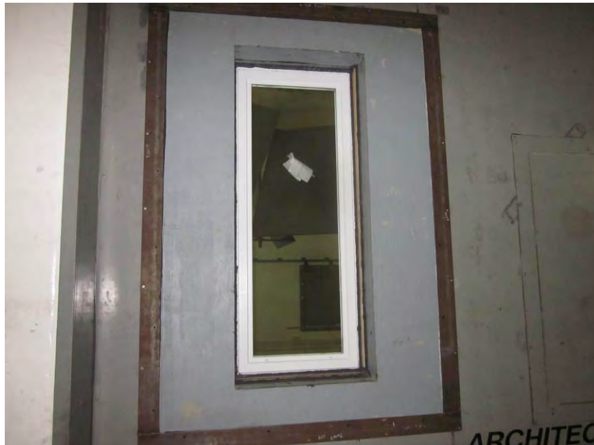
Source Room View of Installed Specimen
